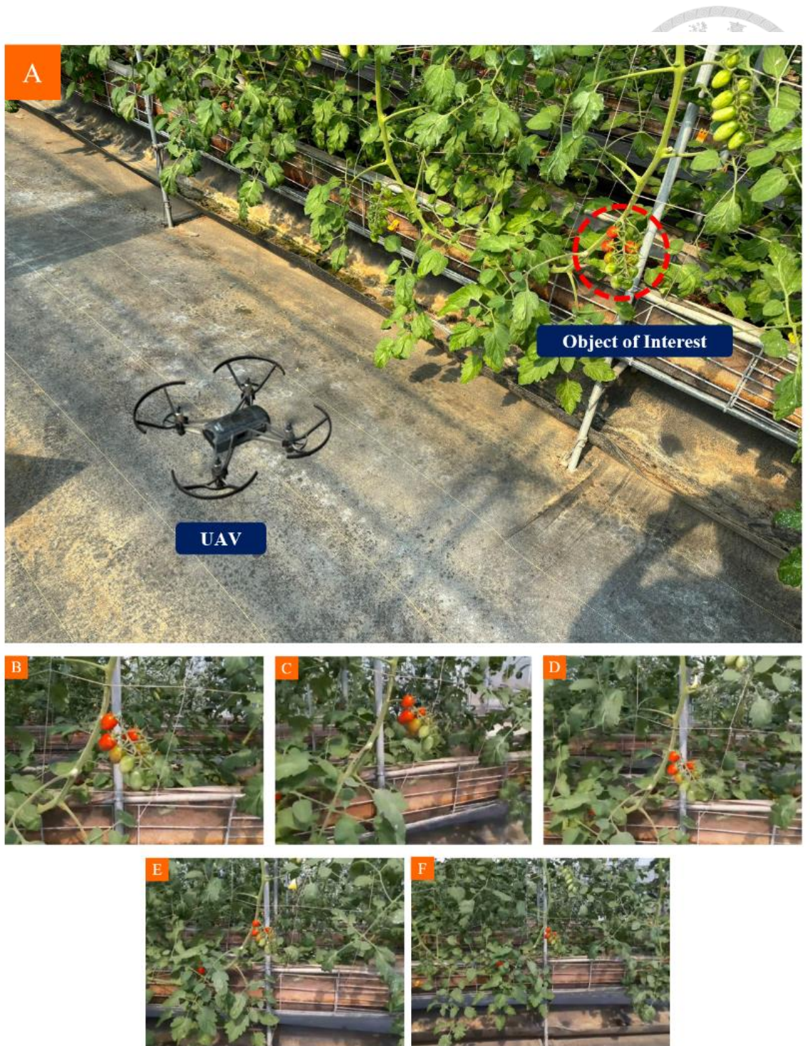
Figure 16. Determination of the Influence of Distance on the Object Detection Performance: (A) Actual Setup; (B) Sample Frame (at 0.2 m OTC Distance); (C) Sample Frame (at 0.4 m OTC Distance); (D) Sample Frame (at 0.6 m OTC Distance); (E) Sample Frame (at 0.8 m OTC Distance); and (F) Sample Frame (at 1.0 m OTC Distance)
