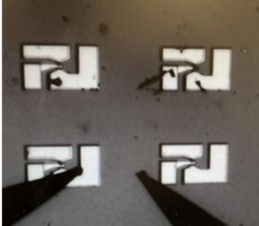
Figure 4.23 OM image of 3 rd lithography (a) Sample 3 (b) Sample 4
