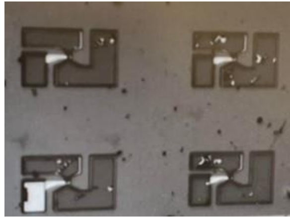
Figure 4.23 OM image of 3 rd lithography (a) Sample 3 (b) Sample 4
