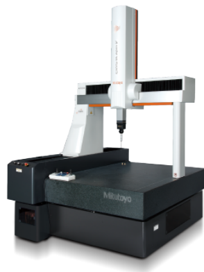
Figure 2.1 A coordinate measuring machine produced by Mitutoyo [6].
