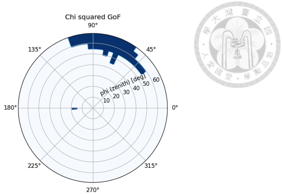
Figure 5.12 \chi^2 goodness-of-fit test, rejected sample data. Null hypothesis is rejected in blue regions.
