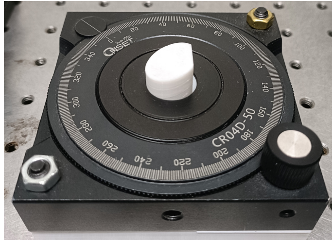
Figure 5.3 A 25° standard block mounted on the rotary stage.
