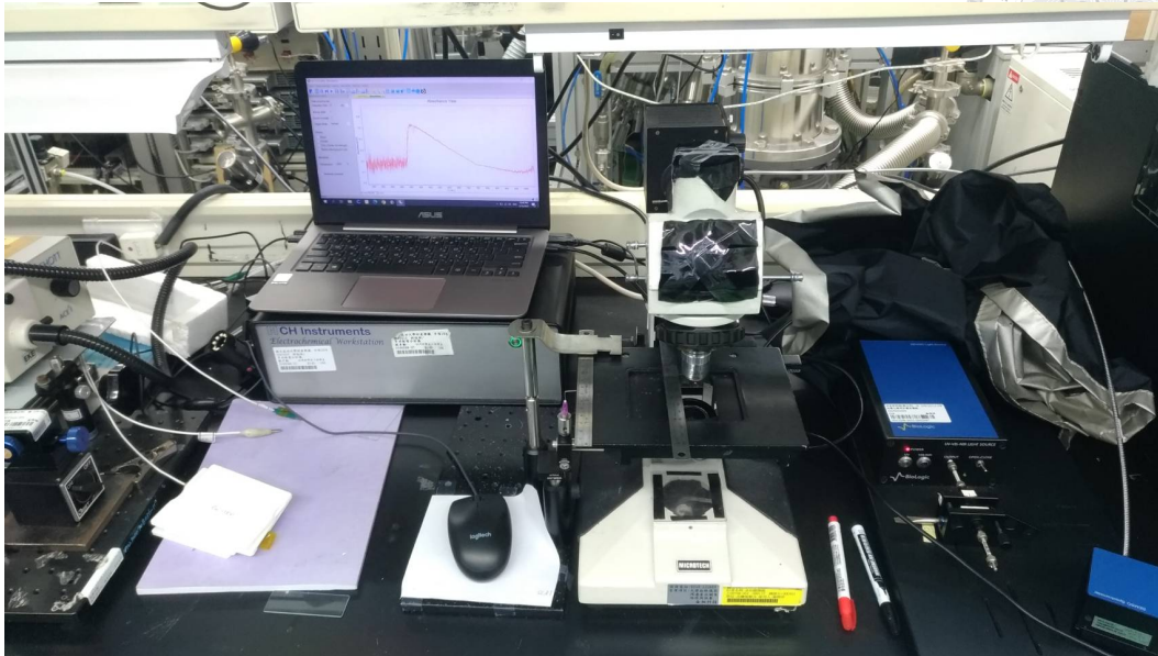
Figure 3.7: The self-made visible light spectrometer in our laboratory.
