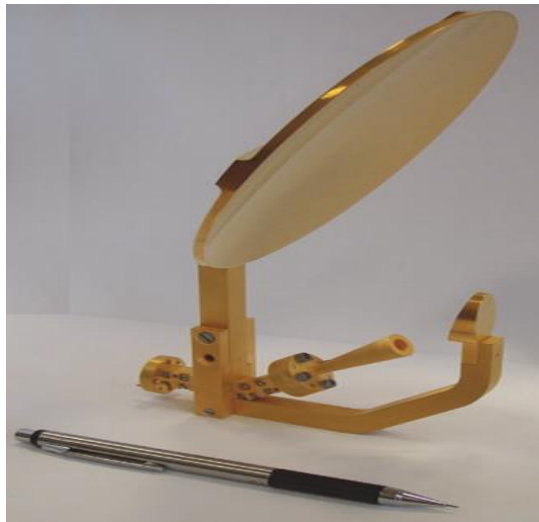
Fig. 2.4 Dual offset cassegrain reflector [4].
