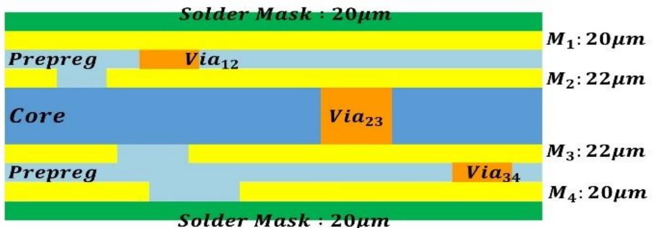
Fig. 3.1 Stack-up representation of the substrate.
