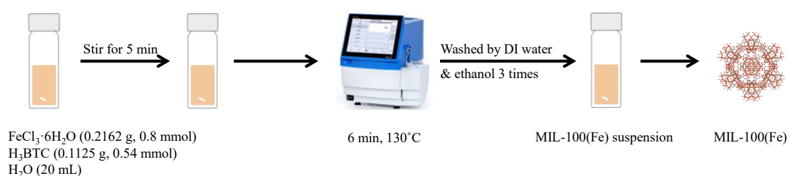
Fig. 4.1. Schematic illustration of the synthesis procedure for MIL-100(Fe).
