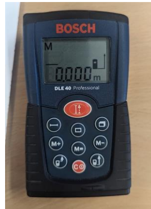
Figure 5.23 : The laser range finder used in experiments
