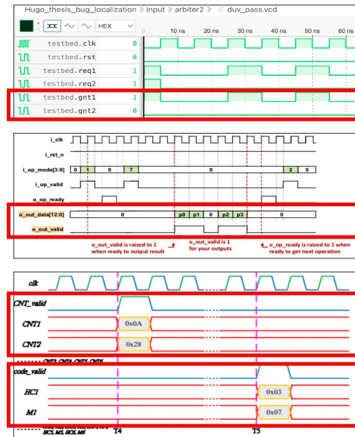
Figure 3.8: The sample waveforms illustrating the output valid signal
