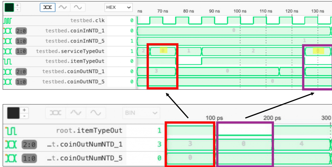
Figure 6.9: The example of comparing the results between the reference model and the DUV (has output valid signals)
