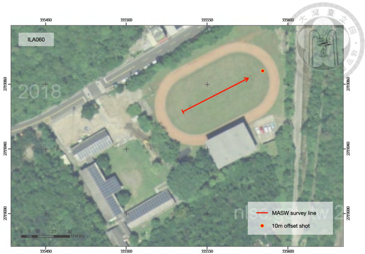
Figure 5.35 The distribution of survey lines in ILA060.
