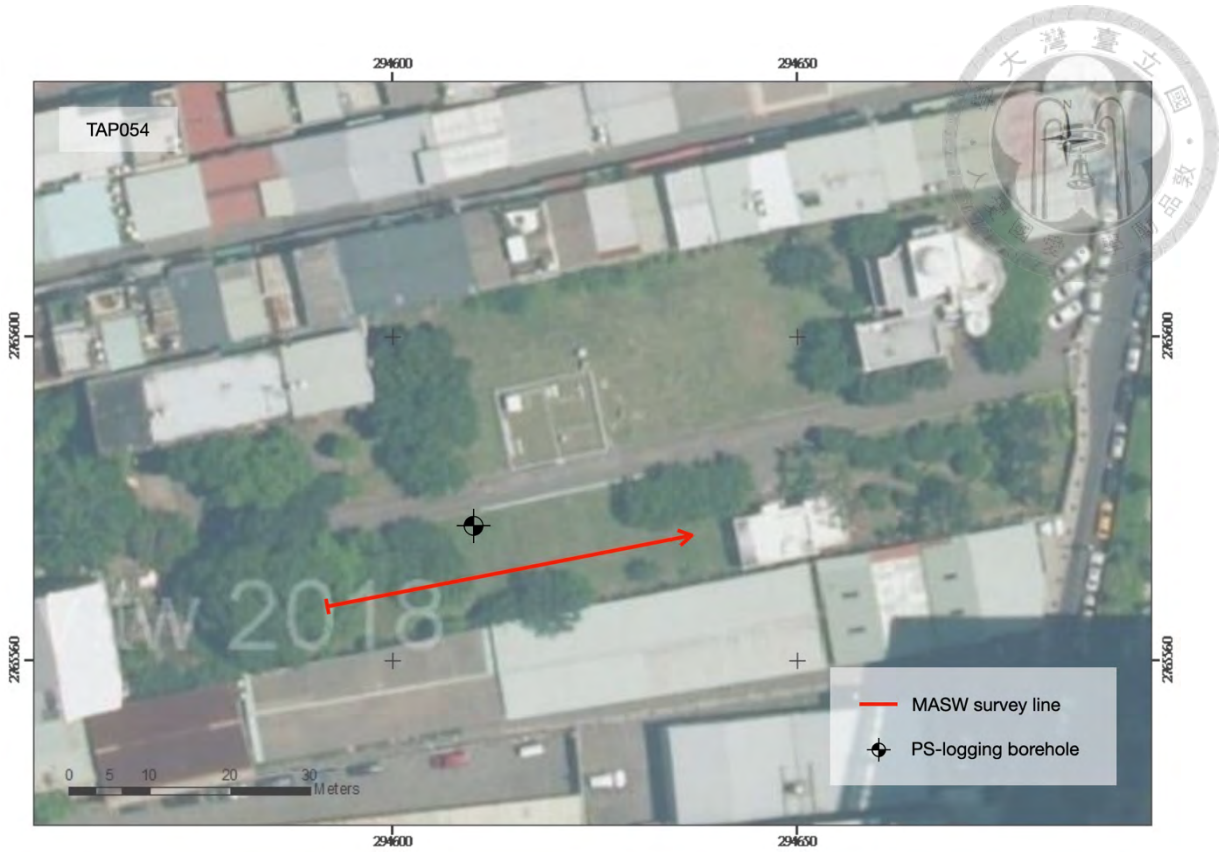
Figure 5.14 The distribution of survey lines and borehole of TAP054.
