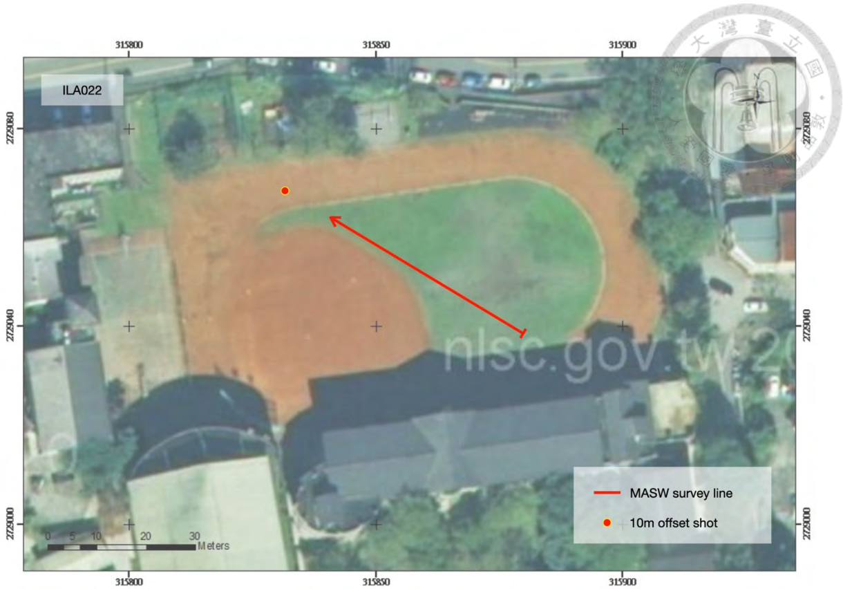
Figure 5.33 The distribution of survey lines in ILA022.
