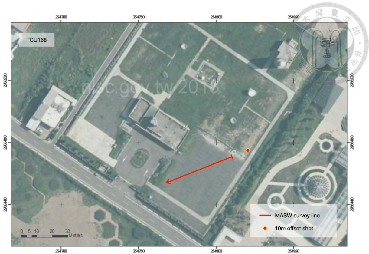
Figure 5.43 The distribution of survey lines in TCU168.
