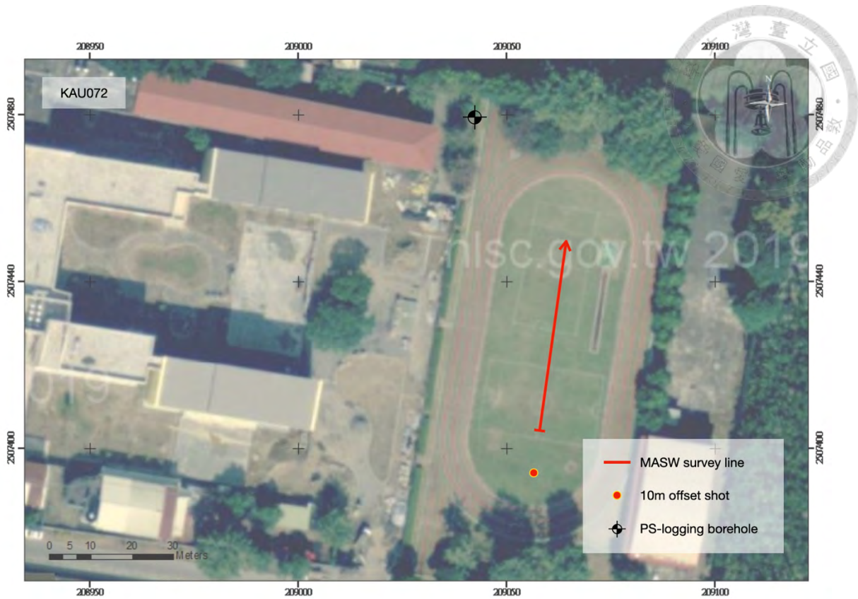
Figure 5.26 The distribution of survey lines and borehole of KAU072.
