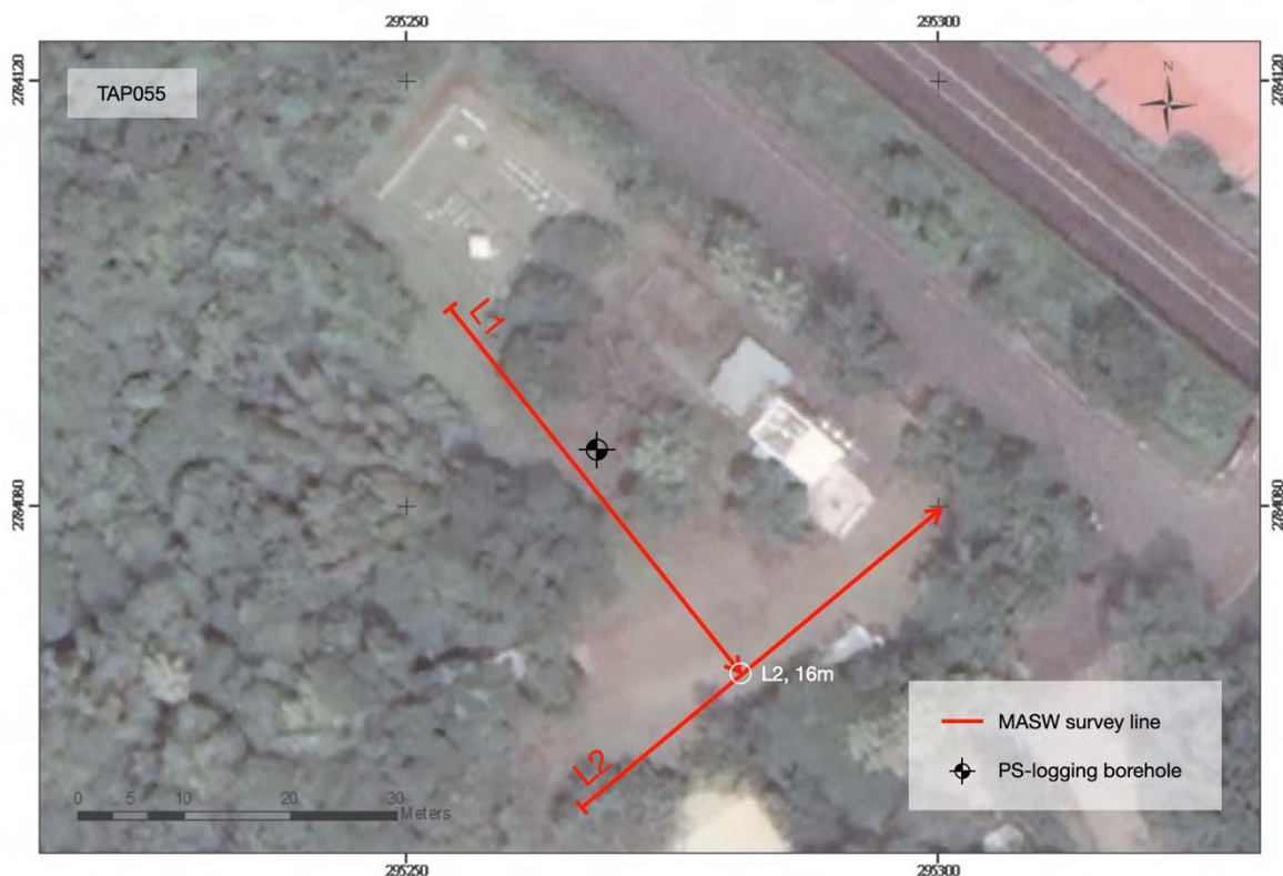
Figure 5.4 The distribution of survey lines and borehole of TAP055.
