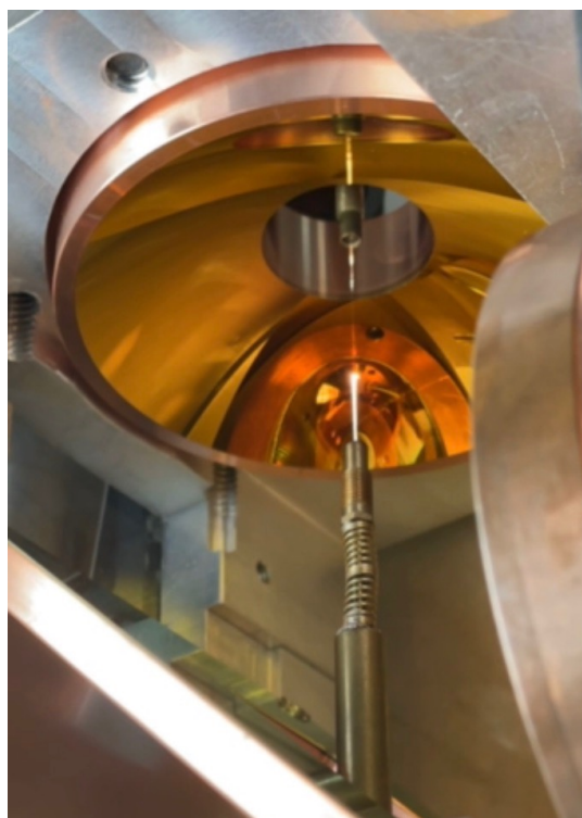
Fig. 3.3. A photo of the growth chamber, illustrating the paraboloidal mirror and the focused CO 2 beam on the source rod.
