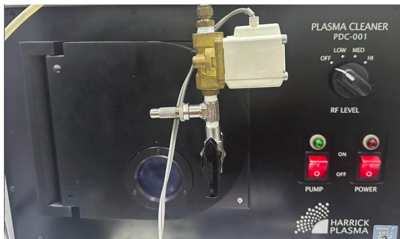
Figure 4-2 Oxygen plasma bonding machine used for device bonding
