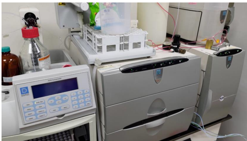
Figure 3.8 DIONEX ICS-3000 at GCRC, National Taiwan University. This is an IC with anion columns, and it measures \text{F}^- , \text{Cl}^- , \text{NO}_2^- , \text{Br}^- , \text{NO}_3^- , \text{SO}_4^{2-} , and \text{PO}_4^{3-} in ppm.
