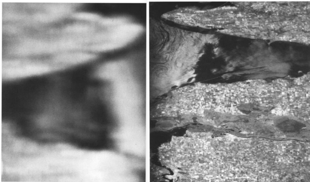
Fig. 3.5. The comparison between amplitude images. Left is the signal from one receiving. Right is improved by SAR technique (derived by Massonnet and Feigl, 1998).
