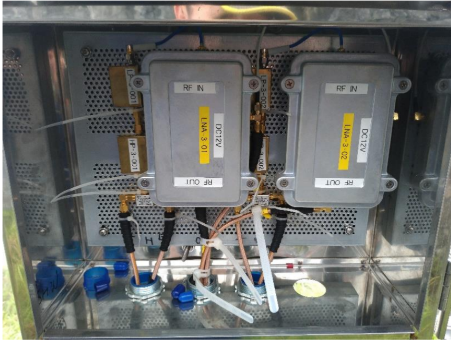
Figure 2.4: FEE modules of TAROGE, including filter and LNA.
