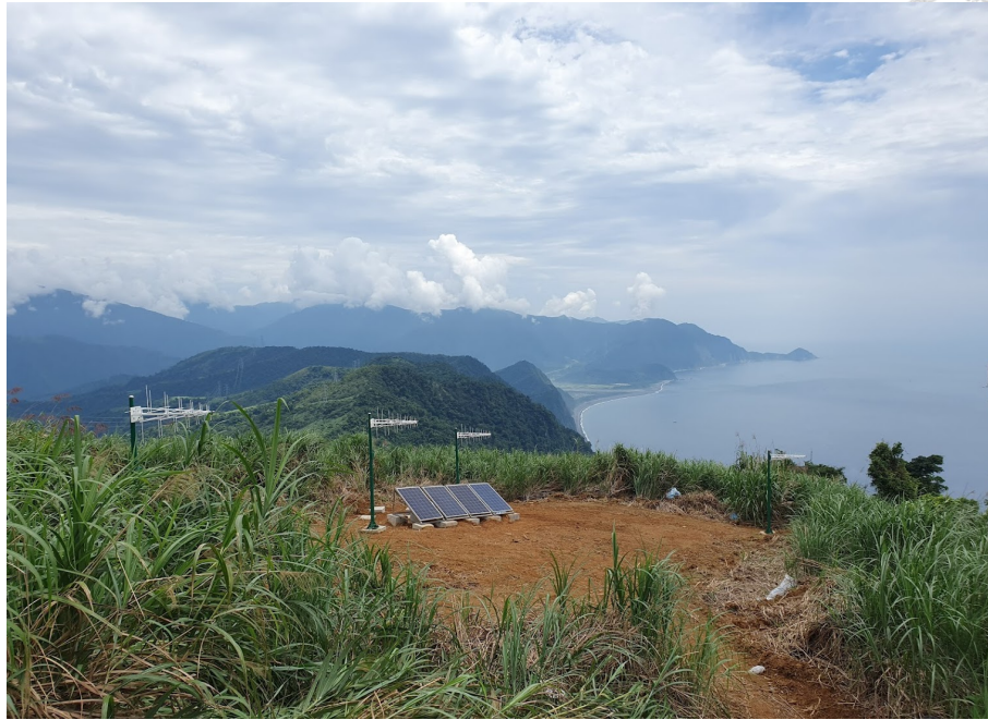
Figure 1.14: TAROGE-4 station, LPDA antennas pointing horizontally to ocean. Adapted from Ref [40].
