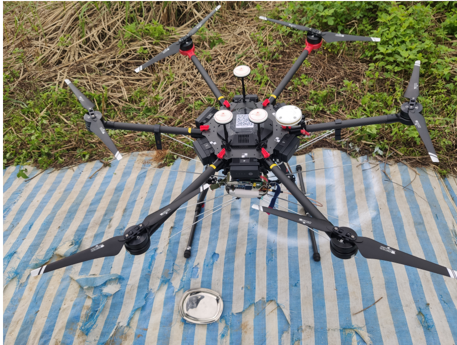
Figure 4.1: Drone-borne pulser system consisting of a high-power impulse generator, a programmable attenuator, a transmitting antenna, and a D-GPS module. This system enables precise calibration of TAROGE-4 by providing well-characterized signals across a wide frequency range and ensuring accurate positional tracking with centimeter-level precision.
