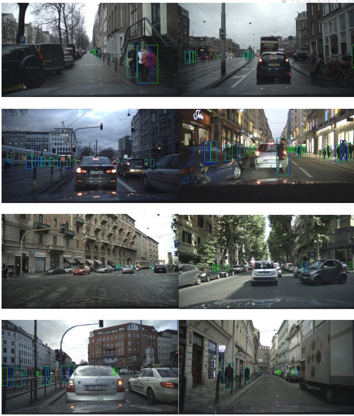
Fig 4.2 Detection result: the green rectangle is our predictions and the blue ones is the ground truths.
