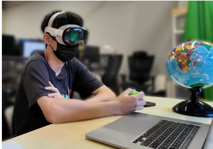
Figure 3.1: The user is wearing the Apple Vision Pro device and is squeezing the ball to trigger the fidgeting interactions.
