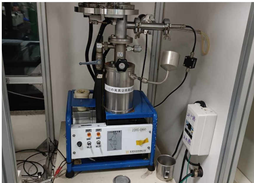
Figure 2.2-2 Thermal evaporator system
