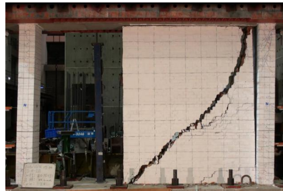
Figure 2-74 Failure condition of Specimen ID-e-1.8 at maximum strength under positive and negative loading (Tung, 2017)
