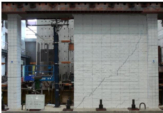
Figure 2-74 Failure condition of Specimen ID-e-1.8 at maximum strength under positive and negative loading (Tung, 2017)
