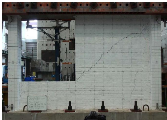
Figure 2-70 Failure condition of Specimen CD-e-1.8 at maximum strength under positive and negative loading (Yang, 2017)
