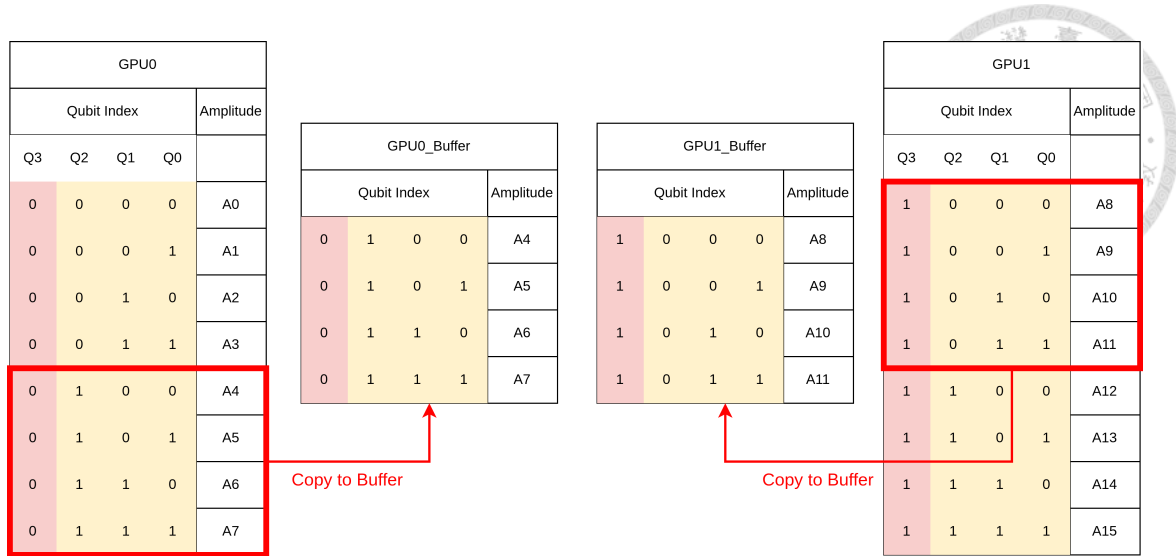
Figure 4.3: Case 1, Step 1: Prepare for Global Data Exchange. The contiguous blocks of amplitudes required by the other GPU (A4-A7 for GPU1, A8-A11 for GPU0) are copied to local buffers.
