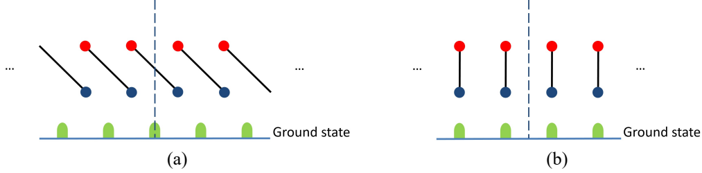
Figure 3.2: The dashed line is the reflection center and the green wave packets represent the charges. (a) By decomposing the ground states, we obtain \psi_c(H_1) = (c_{L+1}^\dagger - c_{L+2}^\dagger)/\sqrt{2} and \psi_c(-H_1) = (c_{L+1}^\dagger + c_{L+2}^\dagger)/\sqrt{2} . Hence, the number of charges located at the reflection center is N_c = 1 for H_1 and -H_1 both. (b) For \pm H_0 , there is no charge located at the reflection center, so \psi_c(H_0) = \psi_c(-H_0) = 0 .
