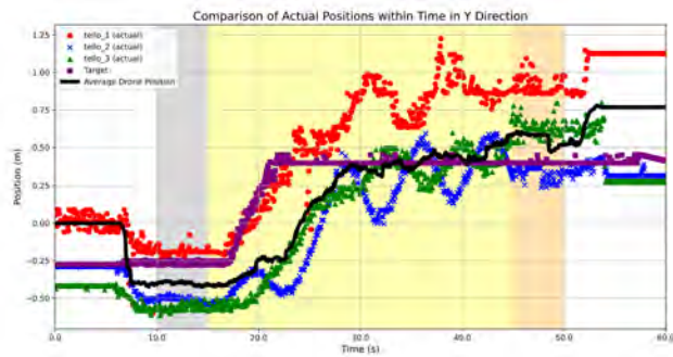
(b) Drone and target positions by RGB camera estimation in Y_W direction.
