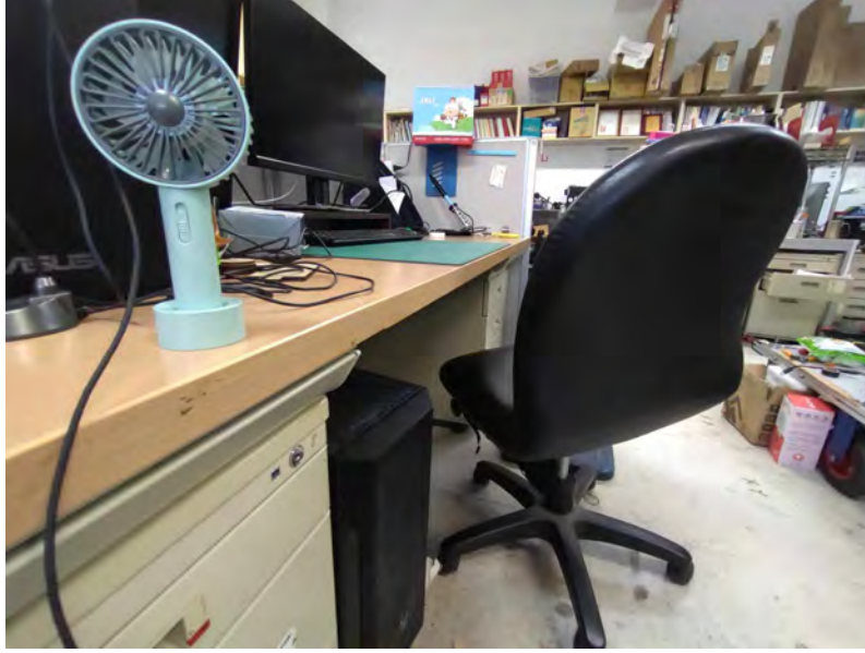
Figure 3.3: Radial distortion on the edge of the image.
