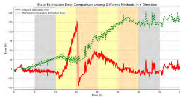
(d) Drone position error by onboard/direct integration of IMU velocity relative to RGB camera estimation in Y_W direction.
