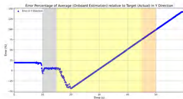
(d) Error comparison of onboard prediction by averaging and estimation by RGB camera in Y_W direction.
