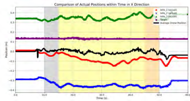
(a) Drone and target positions by RGB camera estimation in X_W direction.
