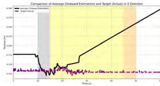
(a) Comparison of onboard prediction by averaging and estimation by RGB camera in X_W direction.
