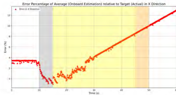
(c) Error comparison of onboard prediction by averaging and estimation by RGB camera in X_W direction.
