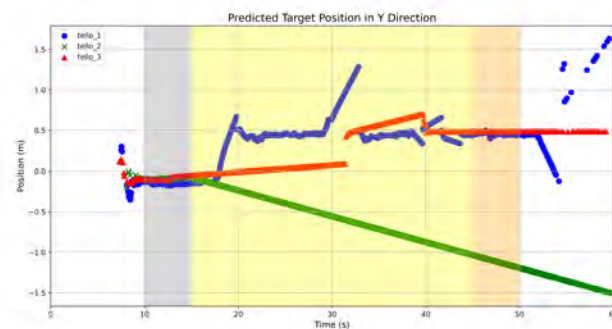
(d) Target positions predicted using curve fitting in Y_W direction.
