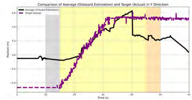
(b) Comparison of onboard prediction by averaging and estimation by RGB camera in Y_W direction.
