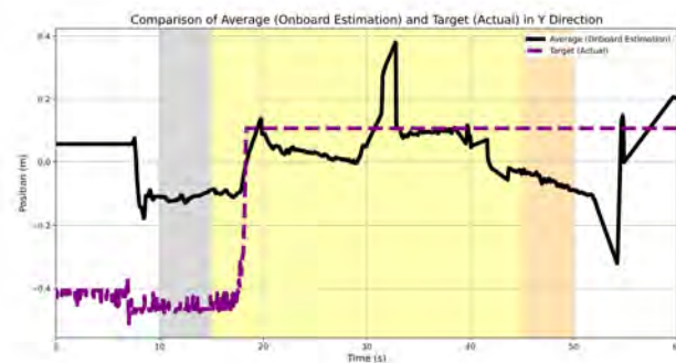
(b) Comparison of onboard prediction by averaging and estimation by RGB camera in Y_W direction.
