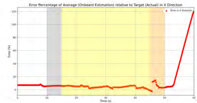
(c) Error comparison of onboard prediction by averaging and estimation by RGB camera in X_W direction.
