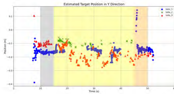
(b) Target positions estimated by the drones in Y_W direction.
