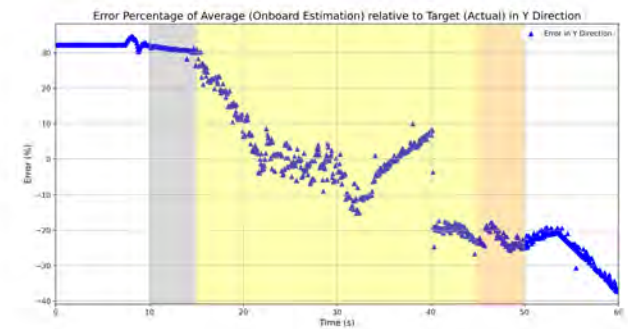
(d) Error comparison of onboard prediction by averaging and estimation by RGB camera in Y_W direction.
