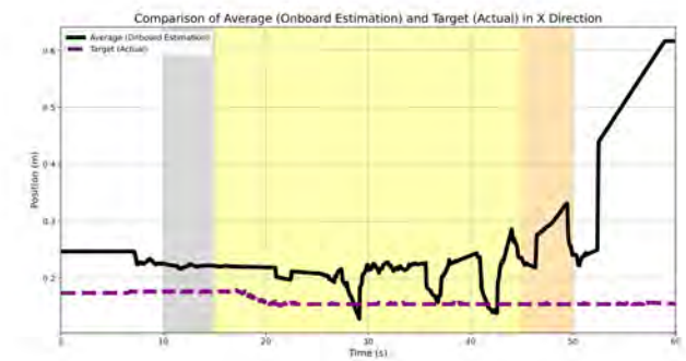
(a) Comparison of onboard prediction by averaging and estimation by RGB camera in X_W direction.
