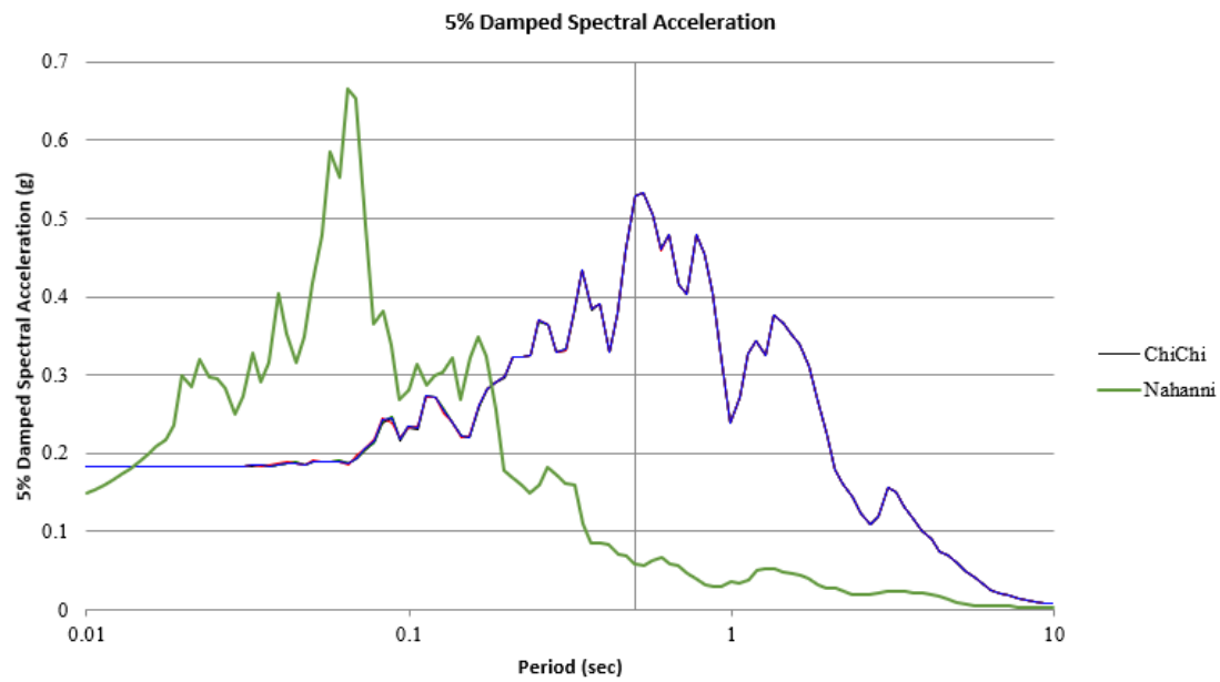
Figure 3.14 Response spectrum of the earthquake used for cyclic softening calculations (DEEPSOIL)
