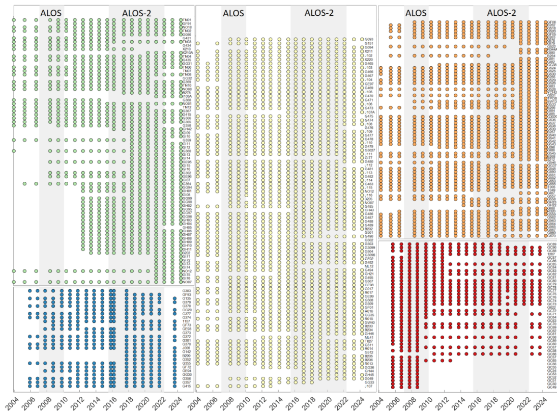
Figure 30. The top panel shows the locations of the five leveling survey lines. The bottom panels display the measure time of each stations on every survey lines, alongside the time periods of the ALOS and ALOS-2 satellite observations.
