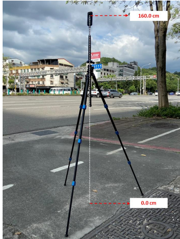
Figure 3-3 Diagram of the Panoramic Camera Setup
