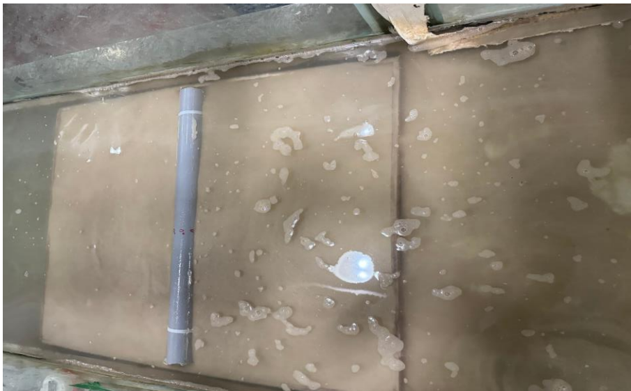
Figure 3.4 Pipeline perpendicular with wave direction ( 90 degrees)
