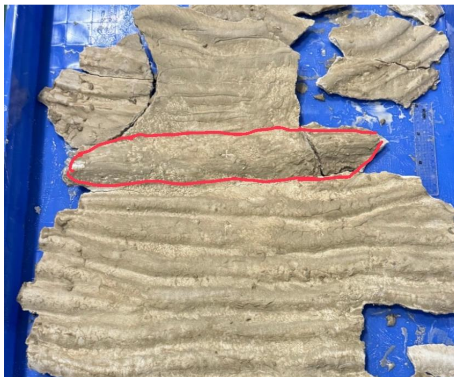
Figure 4.14 Scour found in d90 h40 e0
