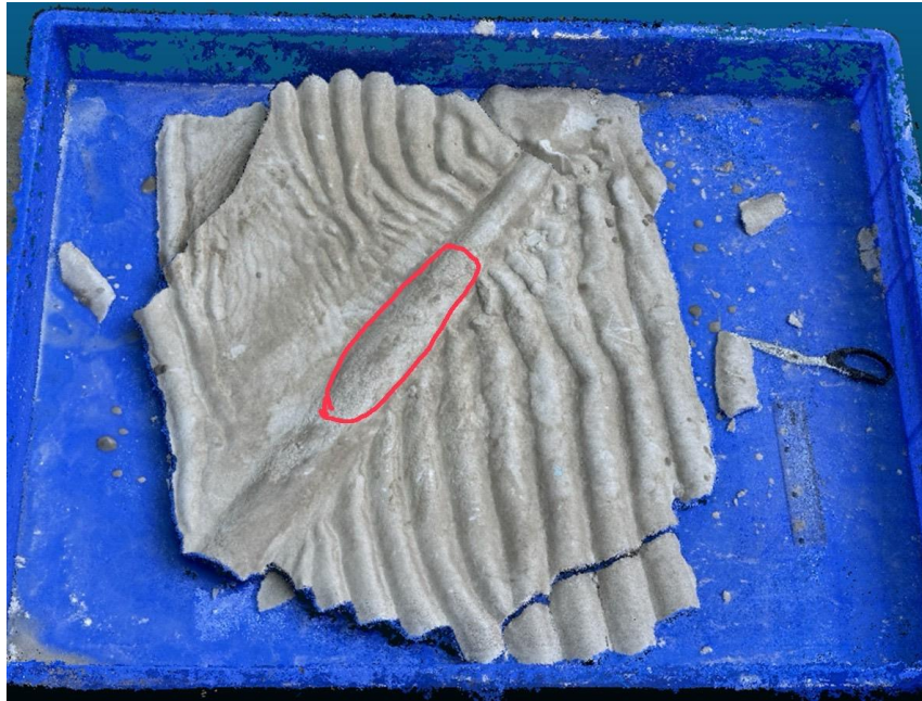
Figure 4.15 Scour found in d45 h40 e0
