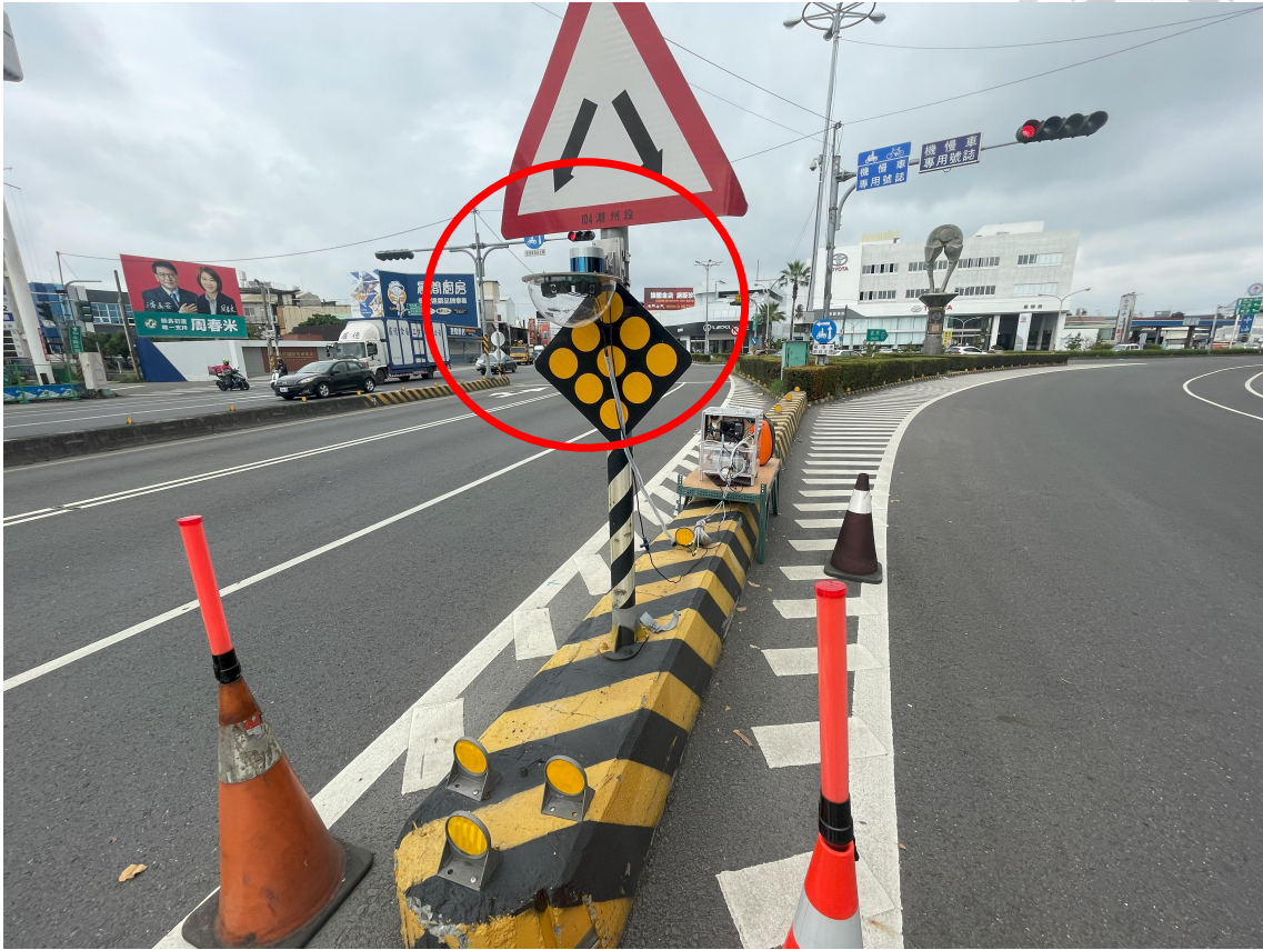
Figure 5.2: Roadside Unit that Collected WAYSIDE Dataset.
