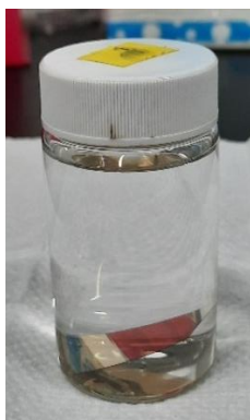
Figure 2-1 The chip is placed in bottles with solvents to lift-off the polystyrene microparticles.
