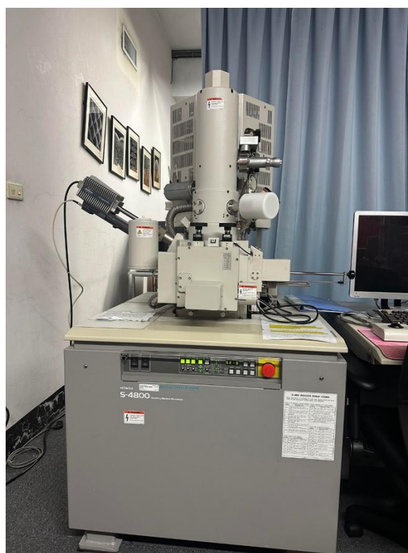
Figure 26: Field Emission- Scanning Electron Microscopy (FE-SEM) Hitachi S-4800 coupled with Energy Dispersive Spectroscopy (EDS)
