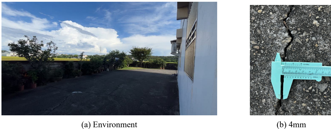
Figure 3.19: For this experiment, we chose a location situated in a shaded area to address lighting issues. To compensate, adjustments were made to the camera focal length and flight altitude. These modifications aimed not only to ensure sufficient lighting and clarity for observing the 4mm-wide crack but also to validate the applicability of our research framework.
