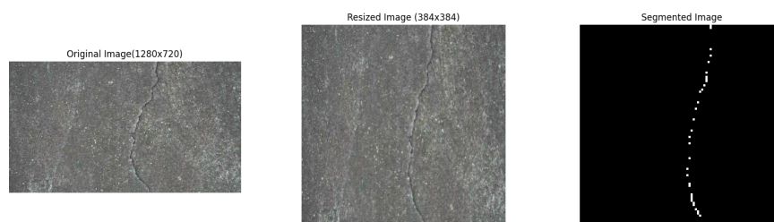
Figure 3.25: At point e , upon obtaining the crack segmentation results, the drone determines forward flight direction using DDQN.
