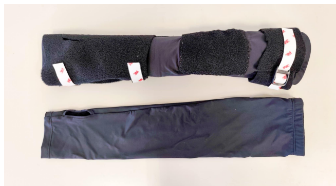
Figure 4.1: Wearable sleeve: (top) modified version, (bottom) original sports sleeve
