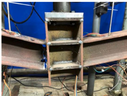
(c) All-welded end of Test
