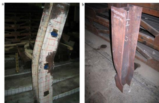
(c) H-Column end of test
