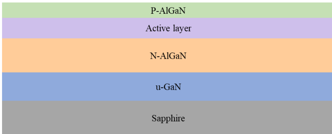
Figure 19 The side view of the epitaxial wafer.
