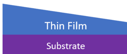
Figure1. 3 Schematic of a wedged-shape sample prepared by wedge deposition, illustrating the gradual thickness variation along the wedge direction.
