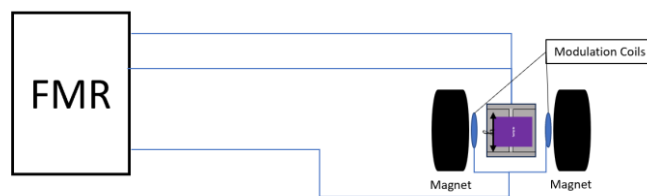
Figure2. 14 Schematic diagram of the FMR measurement setup.
