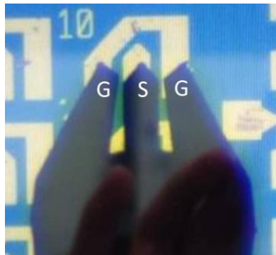
Figure2. 11 Illustration of the probe tips during ST-FMR measurement, with labeled Source (S) and Ground (G).
