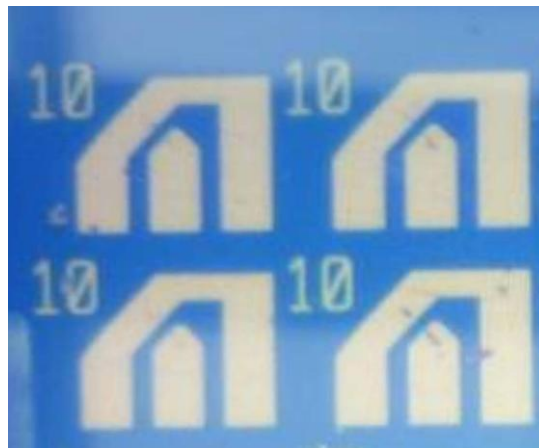
Figure2. 7 Optical image of the final ST-FMR device after fabrication.
