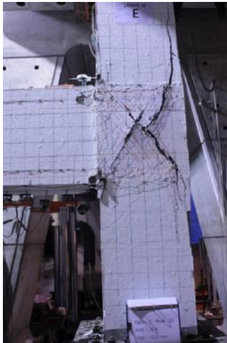
Figure 6-8 Joint LAHHV-SF at failure stage [96]
