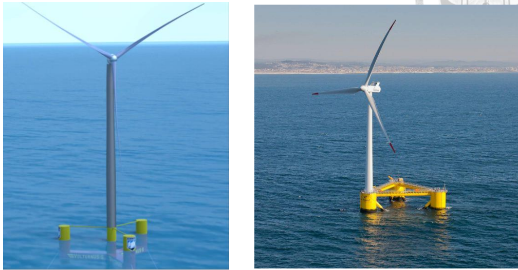
Figure 4: Center-column Platform (Left; VolturnUS [18]) and Off-column Platform (Right; WindFloat Atlantic [19], Courtesy of Principle Power )
