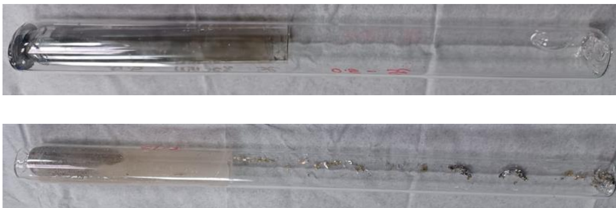
Figure 02.06: Small quartz tube placed inside a sealed larger tube, shown before and after crystal growth
