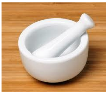
Figure 02.01: Mortar and pestle utilized for material mixing and grinding
