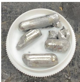
Figure 3.3: Crystal of \text{Sb}_2\text{Te}_3 after sintering process.
