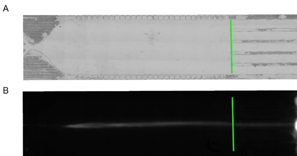
Figure 3-9 The example figures of the fluorescence image measurement under (A) bright field and (B) fluorescent field. The green line represents the measurement location.
