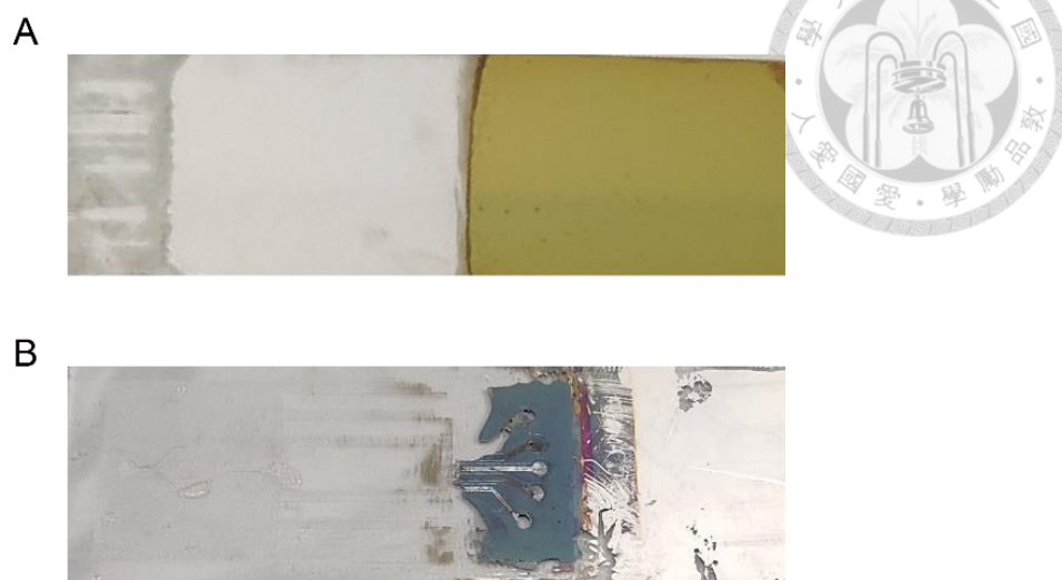
Figure 6-3 Image of the SERS substrate which is an etching by the NaOH (A) Initial state (B) After applying 25 V for 15 minutes.
