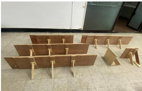
(C) 渠槽分流用木製隔板(背面)
