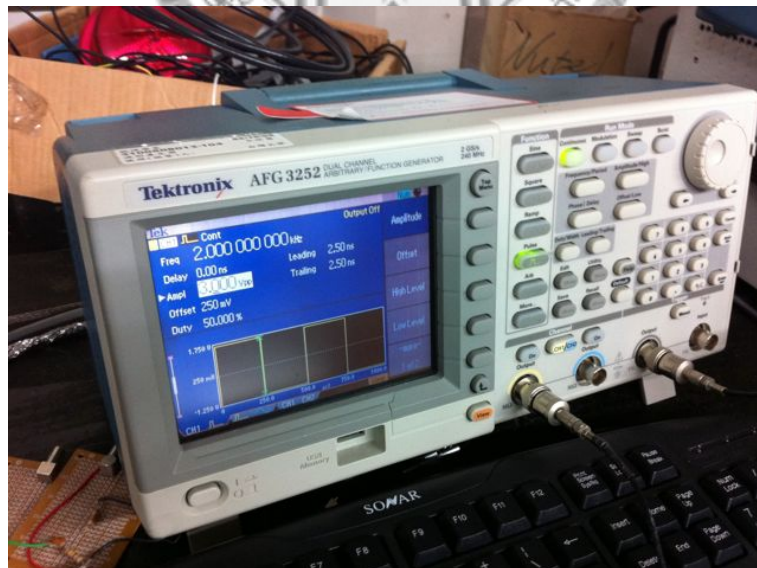
Figure 4.5: Function Generator drives LED and sends a TTL trigger signal to DAQ
