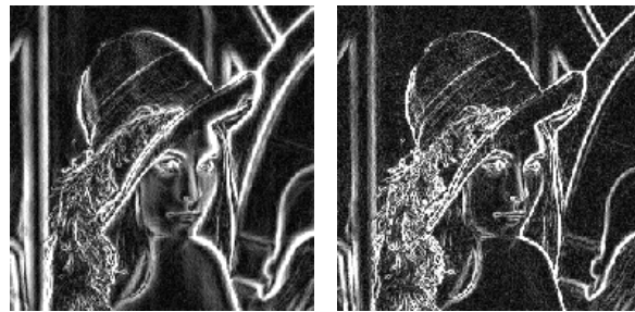
Fig. 2.14 Experiments that use differentiation, the HLT, and the SRHLT ( b=8 ) to detect the edges of Lena image interfered by noise.
