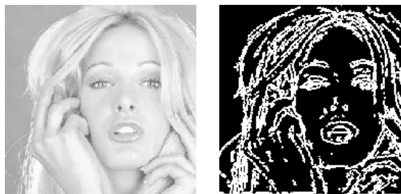
Fig. 2.18 Using the SRHLT ( b = 8 ) to detect the edges of Ken, Shuttle, and Tiffany images. Most of the edges are detected successfully.
