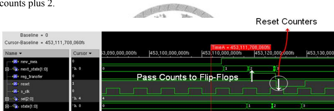
Figure 3.4 The save and reset timing diagram of the control unit.
