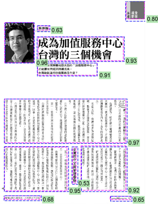
Figure 11. An illustration of accept threshold selection. The groundtruth blocks are marked as magenta and the result blocks are marked as blue. Low MatchScore mostly comes from those small blocks (about 0.8 for logos and 0.6 for footnotes), because a trifling difference (less than 10 pixels) between the two region boundary can result in a large number of percentage of area measure. Thus the smaller blocks tend to have the lower MatchScore. However, this situation does not impede the reading process of users. As a result, we set the accept threshold at 0.6.
