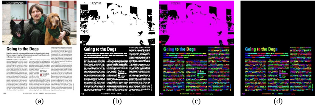
Figure 5. An illustration of the pre-processing steps: (a) Original image. (b) Binarization. (c) Connected component analysis. Components are in different colors. (d) Noise removal and image block pre-extraction.
