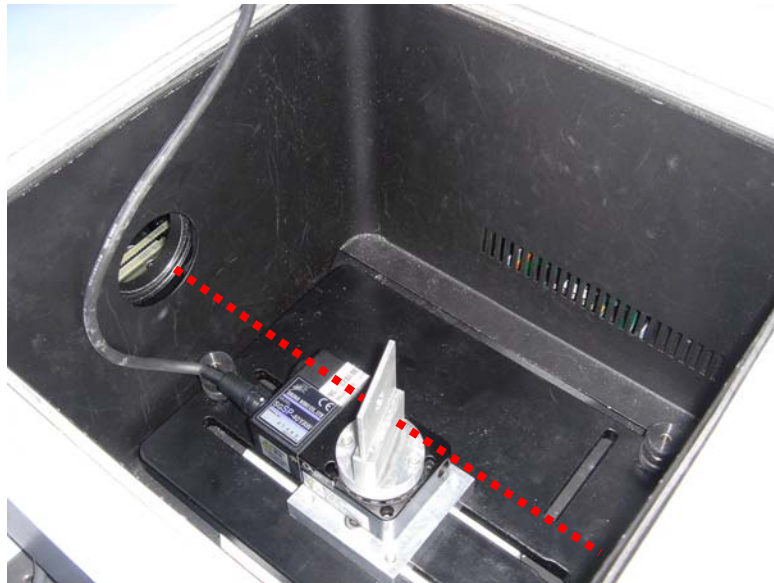
Fig. 2.8 The experiment setup of transmission at incline incidence.
