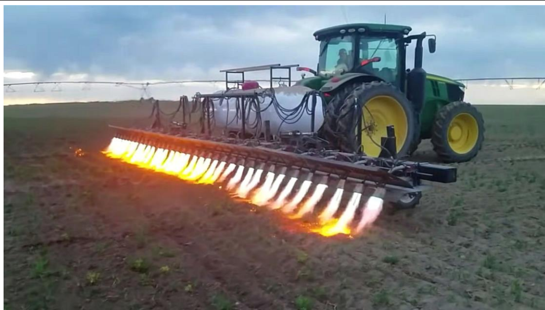
Figure 1.5 The flame trucker is combusting the unwanted weed in preparation stage [80]
