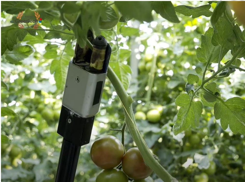
Figure 1.17 The specific robotic system is removing the redundant leaves [26]
