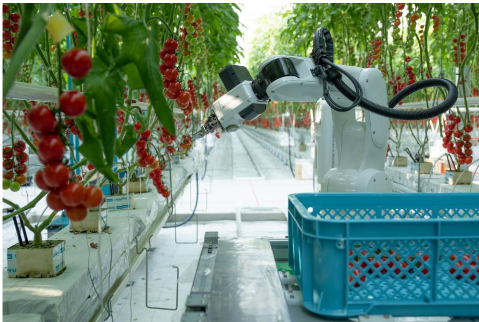
Figure 1.15 A robotic system is cutting the fruit cluster [23]
