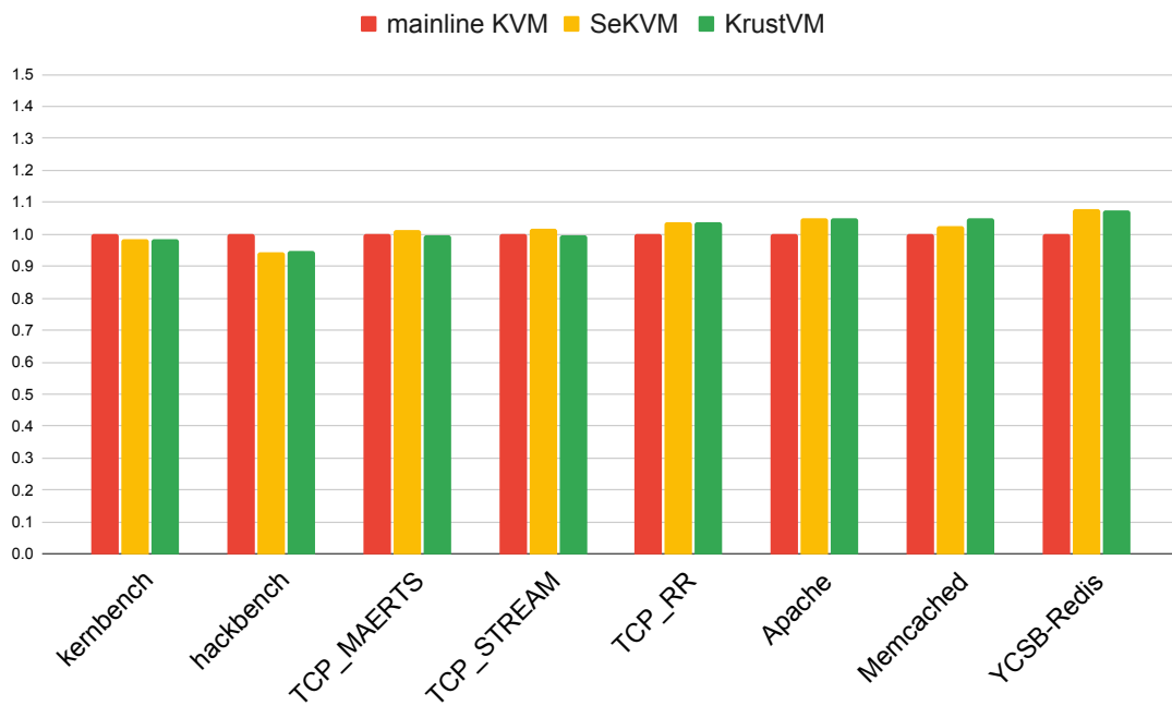
Figure 6.2: Application Benchmark Performance: Overhead normalized to mainline KVM
