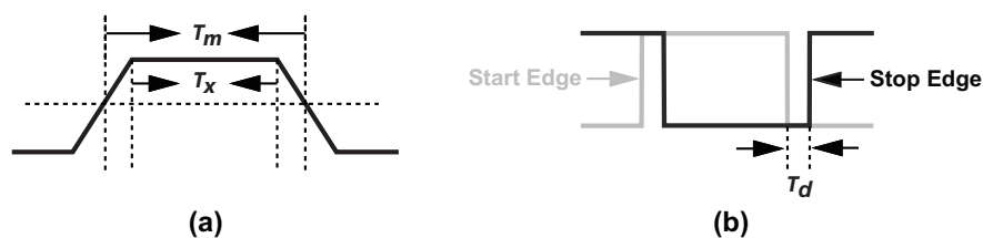
Figure 5.19 Causes of offset error (a) finite rising and falling time and (b) gate delay.
