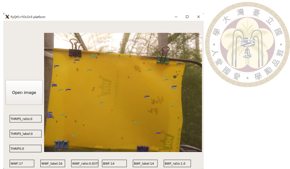
Figure 4.5: Results of object classification and counting using YOLOv5 model with “x6” backbone
