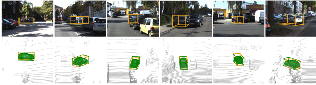
Figure 4.2: Qualitative results of 3D pseudo-bounding boxes. The green shapes are the transformed templates, and the green boxes are the corresponding 3D pseudo-bounding boxes. The orange boxes are the ground truth 3D bounding boxes.
