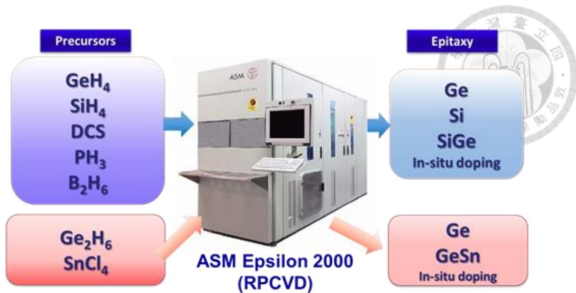
Figure 2-1 An ASM Epsilon 2000 RPCVD system. The original and extended precursor gas systems are used for Si/Ge/SiGe or Ge/GeSn epitaxy.
